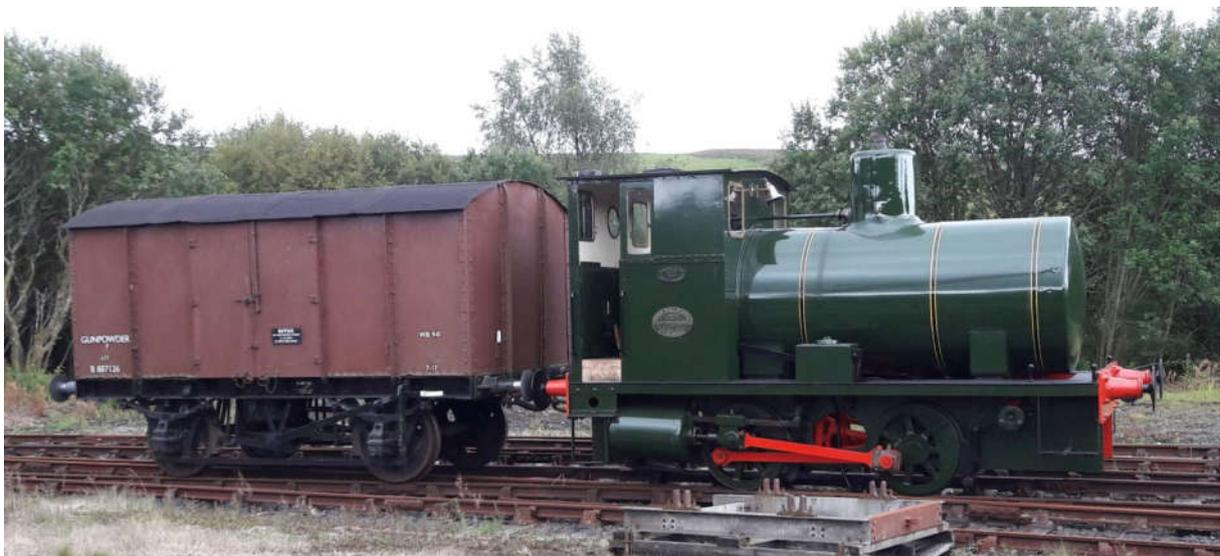
Yes, a fireless steam engine. I know it seems a difficult concept to take on board but the clue is in the word DYNAMITE on the side of the wagon behind the engine. Devil's Porridge also had a fireless the last time I visited them. The engine in the picture is Kilmarnock built. **Ed.**
